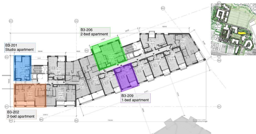
Figure 2: A layout showing the rooms selected for testing within Block B3.
